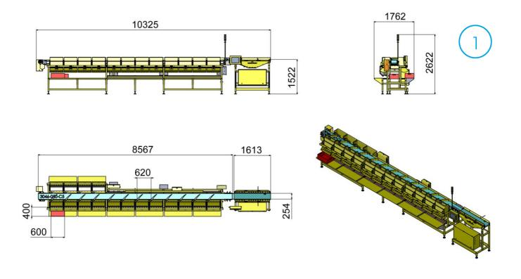
**Batcher Grader, CALIBRA CD 3046** Weighing bridge QUARTZ 1600mm Ejection conveyors 12 stations with buffer and scrap channels
